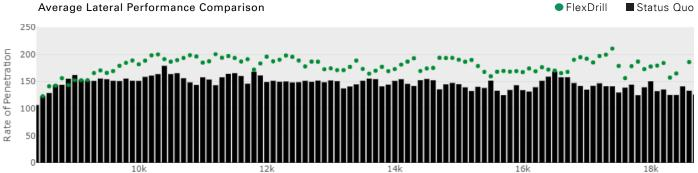
In a foot-by-foot comparison of average ROP, FlexDrill improved the lateral ROP by 21%. This improvement alone translated to a time savings of 8.4 hours.
