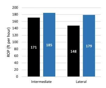
FlexDrill increased the average ROP in both the intermediate section by 8%, and the lateral section by 21%.
