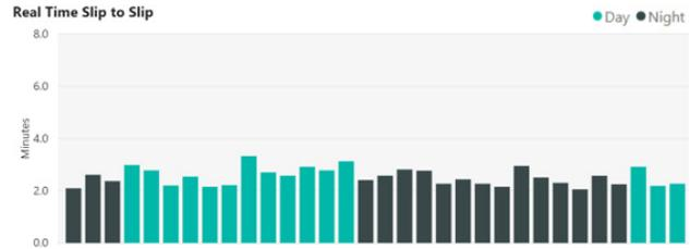
Shortly after FlexConnect utilization, drillers became more consistent. Their slip to slip times were lowered, and inconsistency between crews was significantly reduced.
