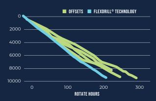
The depth versus time charts displayed above compare the rotating performance of FlexDrill® technology well in the intermediate (left) and lateral (right) sections with relative offsets. The FlexDrill well, displayed in blue, demonstrates far better performance when compared to the average of the offsets.
