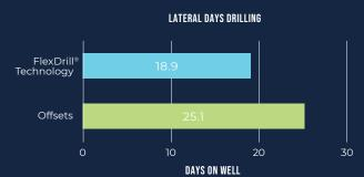
FlexDrill technology's ROP efficiencies contributed to a significant reduction in total days on well when compared with offsets in both the intermediate and lateral sections.
