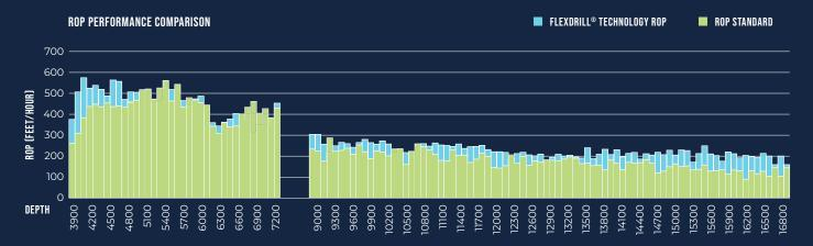
Comparing average ROP for the three wells drilled with FlexDrill® technology as opposed to the standard well, the H&P wells were drilled an average of 40 feet per hour faster than the standard well at the same depth.
