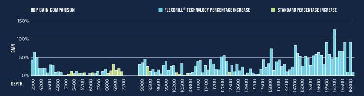
This chart shows the frequency at which the FlexDrill® technology well had an increased ROP when compared to the standard well. The frequency of the blue bars indicates a FlexDrill® technology ROP percent increase, which occurred throughout 83% of the total footage drilled. The frequency of the green bars indicates the standard well's ROP percent increase, which happened during only 17% of the total footage drilled.
