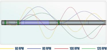
FIGURE 2: MIN/MAX DISPLACEMENT RELATIVE TO CRITICAL SPEED (AMPLITUDE OF VIBRATION)
