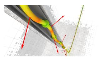
FIGURE 1: ADVANCED 3D VIEWER: HIGH LEVEL OF BUCKLING ALONG LANDING String while Rih with Liner in 3D deepwater well
