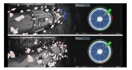
AUTOSLIDE<sup>®</sup> IS A SUITE OF DRILLING SERVICES THAT AUTOMATES THE CONTROL of surface equipment and steerable mud motors to optimize sliding in deviated and horizontal well drilling.
